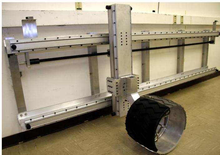
**Figure 12: Tire Surface Wear Life Test Setup**
