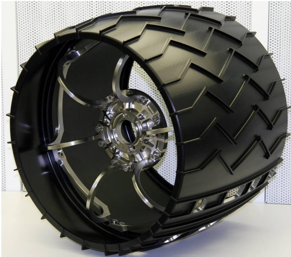
**Figure 6: Flight Design: MSL Wheel Assembly**
