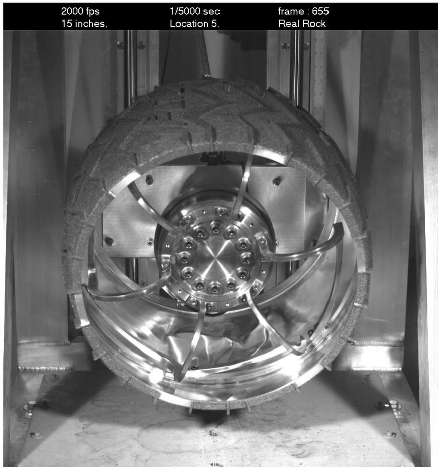
**Figure 16c: Tire Deformation During Mid-Skin Impact**
