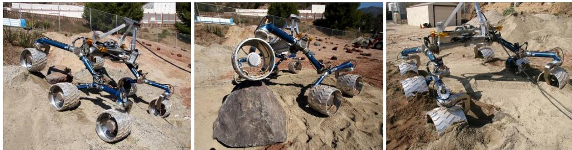
**Figure 11: Traverse Testing of Full-Scale Mobility System**
