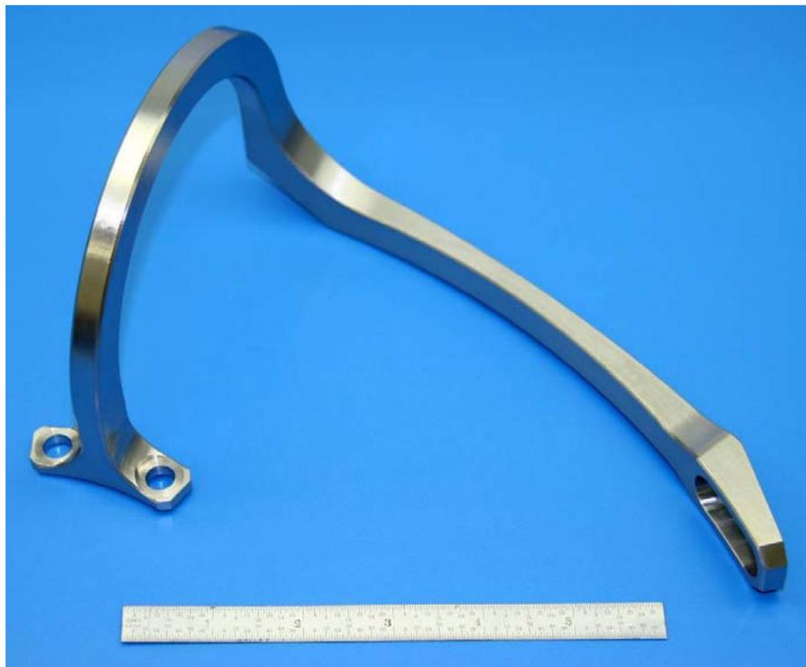
**Figure 7: Flight Design: MSL Wheel Flexure**
