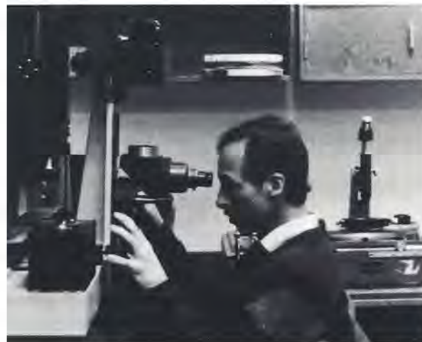
Dave Balam searches for asteroids with the blink comparator. The machine "blinks" rapidly to and fro between two photographs taken hours apart. It's easy to detect an asteroid by its motion. Photograph: Charles Card
