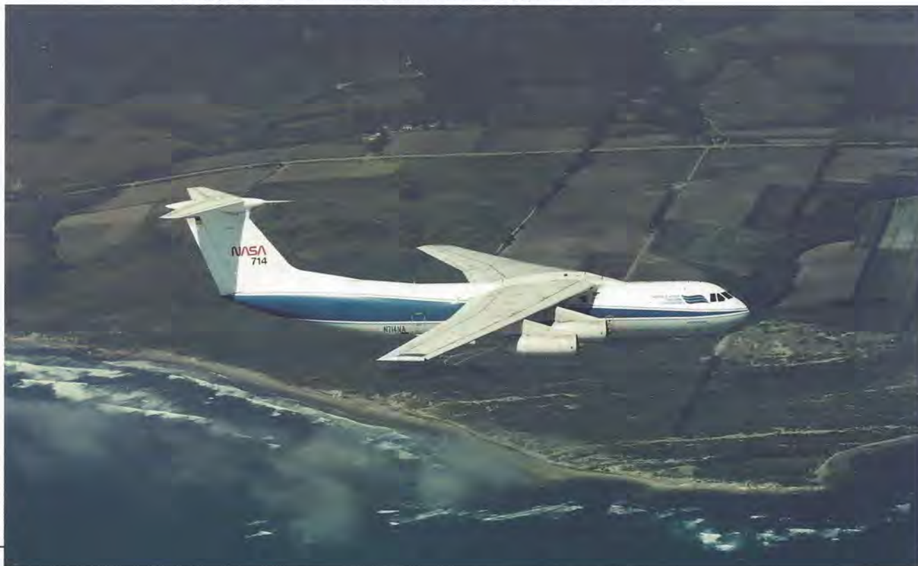
NASA's Kuiper Airborne Observatory carries instruments and astronomers high above Earth's interfering atmosphere. Among the discoveries made from the observatory are the rings of Uranus and the atmosphere of Pluto. Photograph: NASA/Ames Research Center
