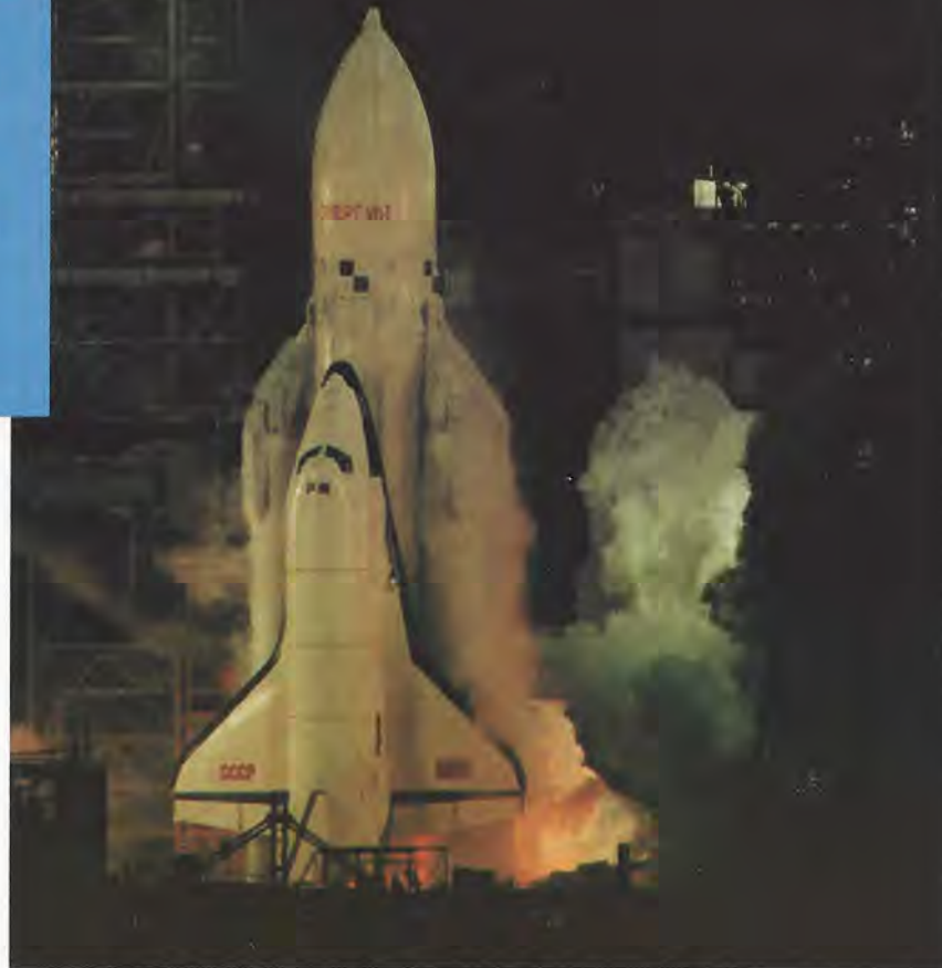
The multi-purpose launch vehicle Energia carried the Soviet space shuttle Buran on its maiden flight on November 15, 1988. With its central fuel tank and strap-on boosters, Energia resembles the American shuttle launch system, but there are significant differences; most important, Energia can carry either a shuttle or a heavy-payload module to Earth orbit and beyond. This heavy-lift capability has led some American space observers to suggest that instead of developing another shuttle-based launch system, NASA might buy Energia launches from the Soviets. In fact, a Houston-based attorney has secured the rights to market Proton and Energia launches.
