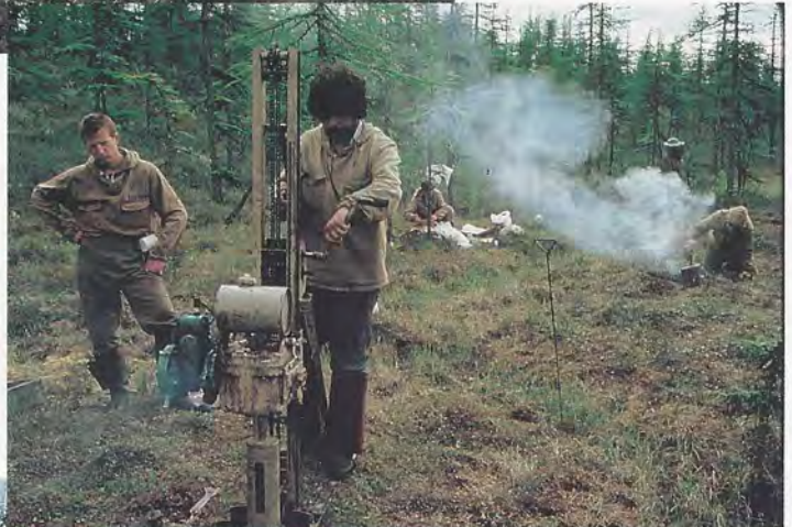
To obtain uncontaminated samples of permafrost, we used a special drill. Here David Gilichinsky is drilling into the permafrost near the Kolyma River exposure seen in the photo above. Dr. Gilichinsky is a leading authority on permafrost and drilling operations.
