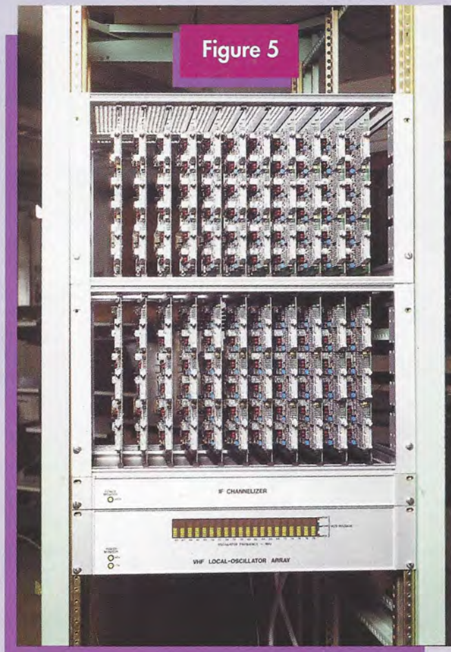
Figure 5. BETA is growing! The electronic equipment shown here converts the analog radio signals received by the antennas to a stream of 240 million numbers (bytes) per second, in preparation for the digital spectrum analyzer and signal recognizer, which together perform about 25 billion operations per second (25,000 MIPS). Photograph: Paul Horowitz
