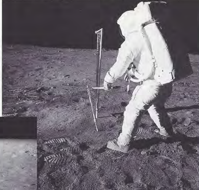
Apollo 11 (above): Buzz Aldrin drives a core tube into the lunar soil and retrieves a sample for return to Earth. In the background is the Solar Wind Composition experiment, which he had just deployed. Even on this first mission to land humans on the Moon, astronauts completed several scientific experiments. Photograph: Neil Armstrong, NASA
