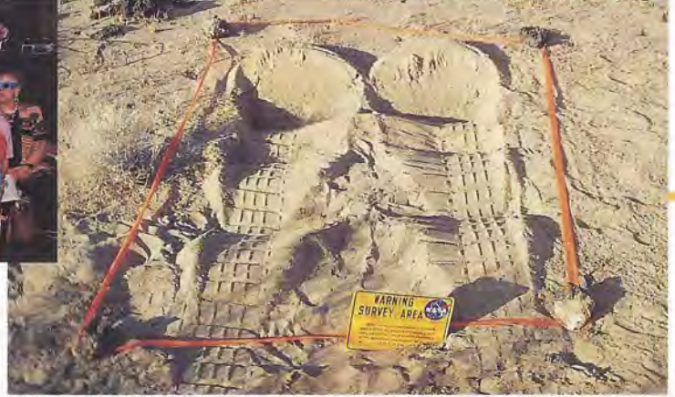
Even tracks in the sand yielded data for the science teams. At this site they were measuring the digging potential of one pair of the rover's six wheels. Photograph: Wade Sisler, NASA Ames Research Center
