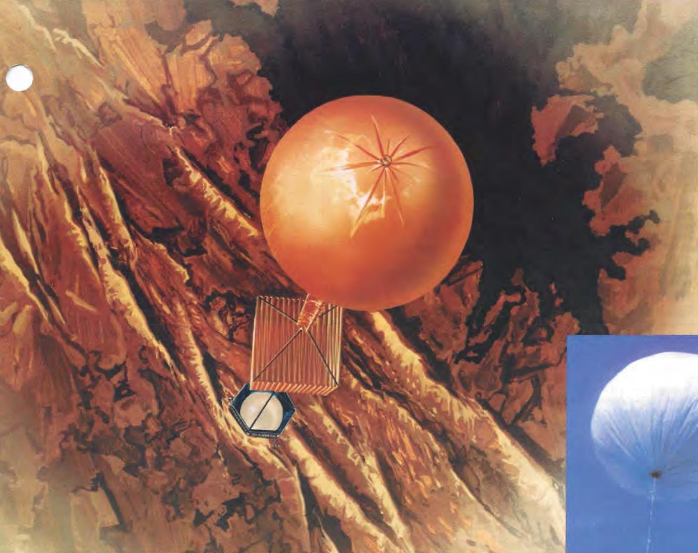
*Above: The Venus Geoscience Aerobot, a descendant of the VEGA balloons, would repeatedly travel between the cool upper atmosphere, with temperatures around 0 degrees Celsius (32 degrees Fahrenheit), to the quite nasty lower atmosphere, where it would have to endure temperatures up to 460 degrees Celsius (about 860 degrees Fahrenheit). Illustration: JPL/NASA*
