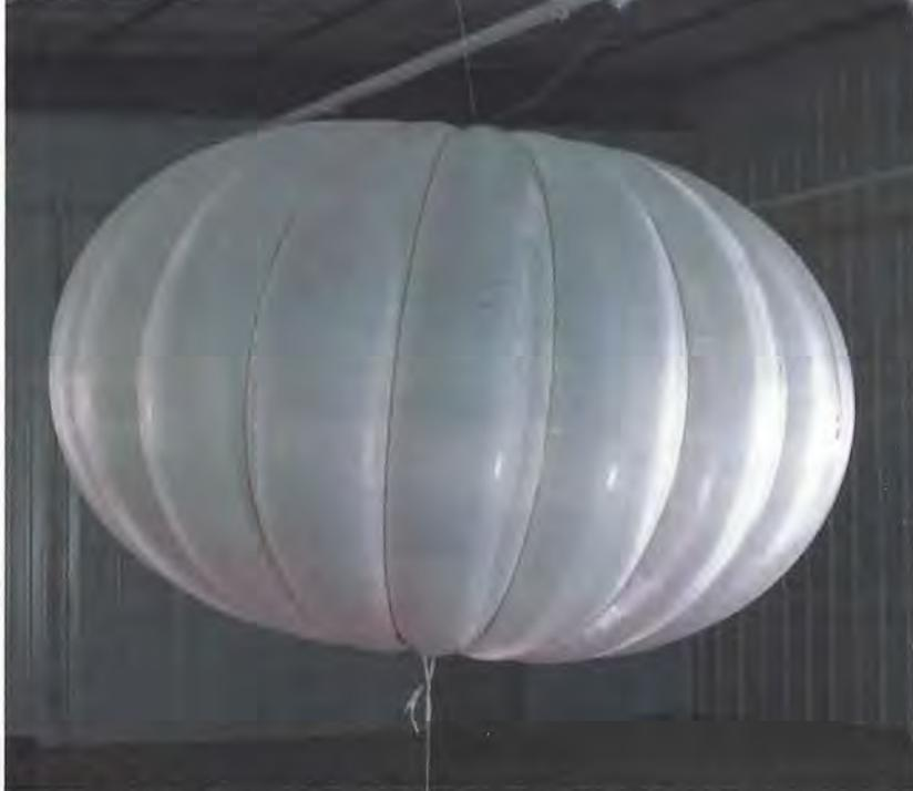
*Above: NASA is testing various designs for ultra-long-duration balloons in Earth's atmosphere, and some of these superpressure designs might someday fly on Mars. This is the pumpkin design from the space agency's Wallops Flight Facility. Photo: NASA*
