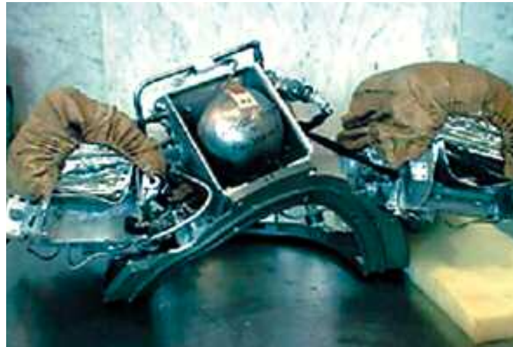
Shown here is the test spacecraft's damaged and deformed mounting platform, with the solar sail blades packed on top. The deformation was caused when the craft's inflatable reentry system engaged inside the capsule and pushed on internal components. Flight unit backups of the sail blades and the damaged tanks and structures were used to repair the test capsule. Image: Babakin Space Center
