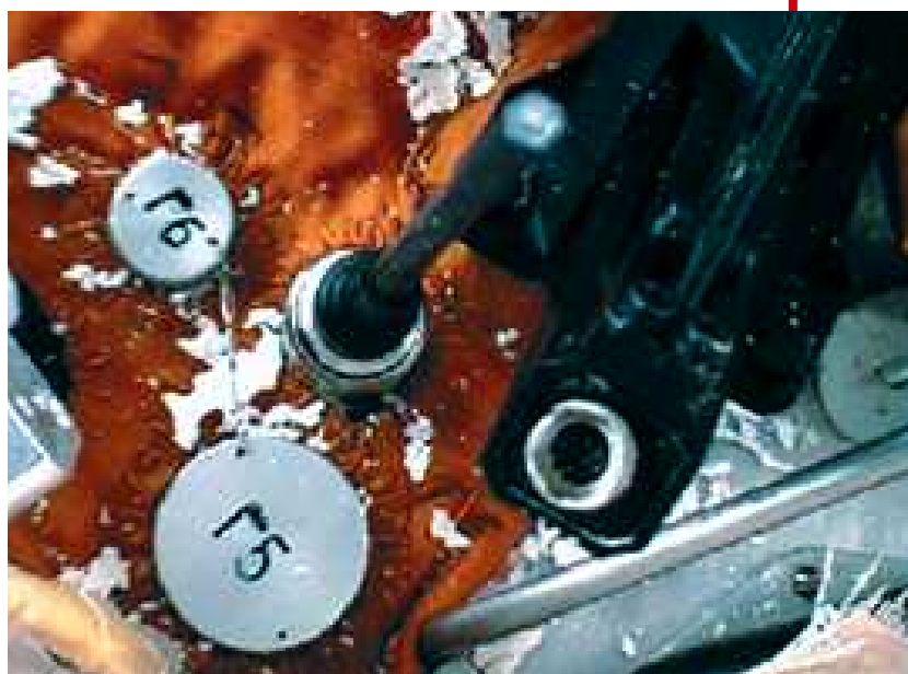
Seen here is the site of the short circuit that damaged the Cosmos 1 test spacecraft. In view is the G5 ground support connector, with its metallic cap installed over the connector pins. The team believes this cap shorted across several pins, causing the descent computer to begin its sequence.
