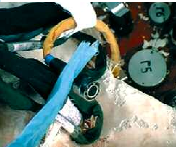
This broken cable was meant to pass data from the camera to the spacecraft's computer. All wiring and all damaged connectors were replaced for the sub-orbital test flight.
