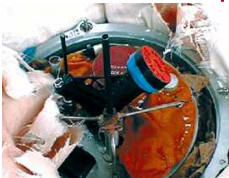
This is the upper part of the instrument container, showing the camera with its "remove before flight" lens cap (red) and shredded inflatable reentry material on the left. Images: Babakin Space Center
