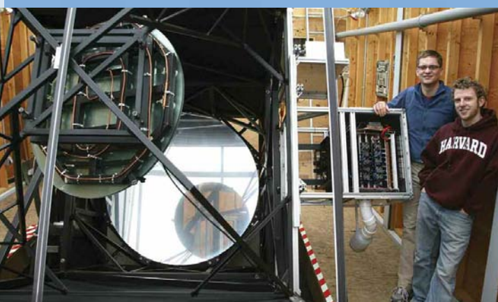
We are looking down into the telescope. The large mirror is the 72-inch primary mirror. It reflects light to the 36-inch secondary mirror, which we see the back of here (it's the circular object at left). Light is then reflected to the detectors, which, along with the electronics, are in the cubelike structure at right, next to graduate students Andrew Howard (left) and Curtis Mead. Photo: Paul Horowitz
