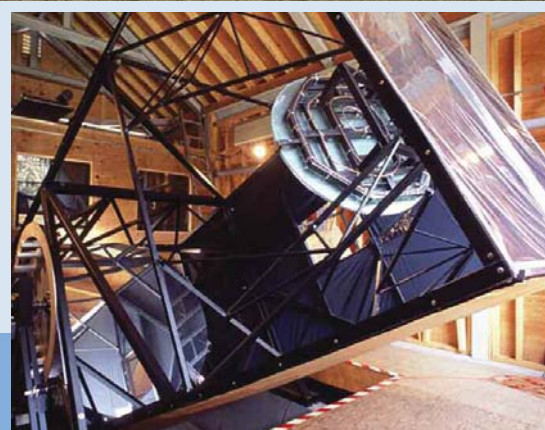
The telescope with an open frame (in operation, the sides will be covered and the top cover, shown here, will be removed). Note the 1.8-meter primary mirror at lower left as well as the back of the 0.9-meter secondary mirror at upper right.
