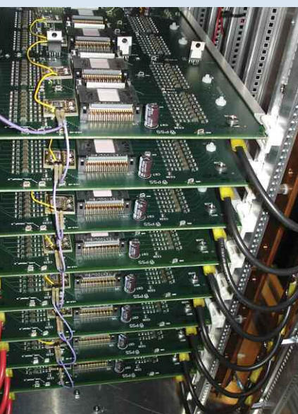
These are the eight boards that hold the 32 custom-designed PulseNet chips. These chips allow the telescope system to process the same amount of data as that in all of the world's books in print—every second!
