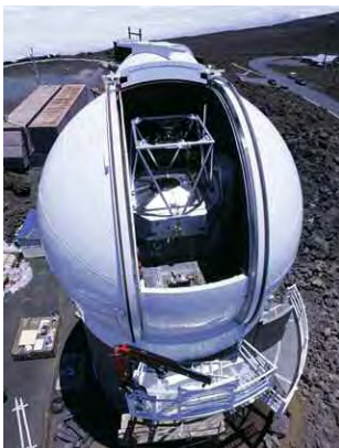
The Pan-STARRS 1 (PS1) telescope, visible inside its dome on top of Maui's Haleakala peak, will use its 1.4-gigapixel camera to find distant asteroids headed for Earth.
