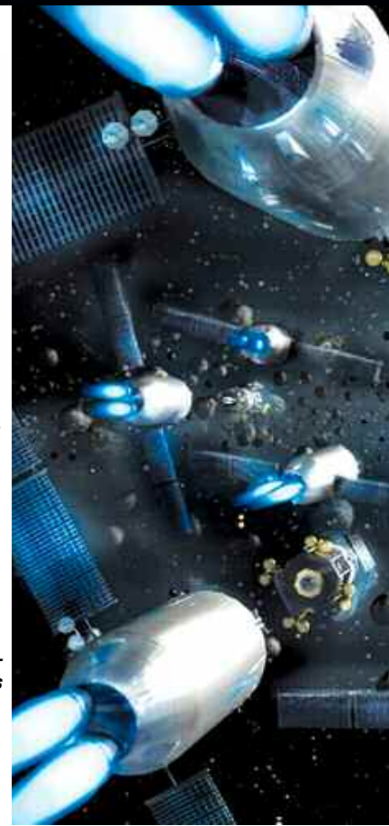
A fleet of MADMEN (Modular Asteroid Deflection Mission Ejector Node) spacecraft swarms a menacing near-Earth asteroid. The small spacecraft will land on and eject mass from the body and thereby alter its trajectory. This illustration was part of a 2003 study on asteroid deflection by SpaceWorks Engineering for NASA’s Institute for Advanced Concepts (NAIC). Illustration: Nathan Phail-Liff, Alien in the Box. Copyright © 2003 SpaceWorks Engineering, Inc. (SEI)
