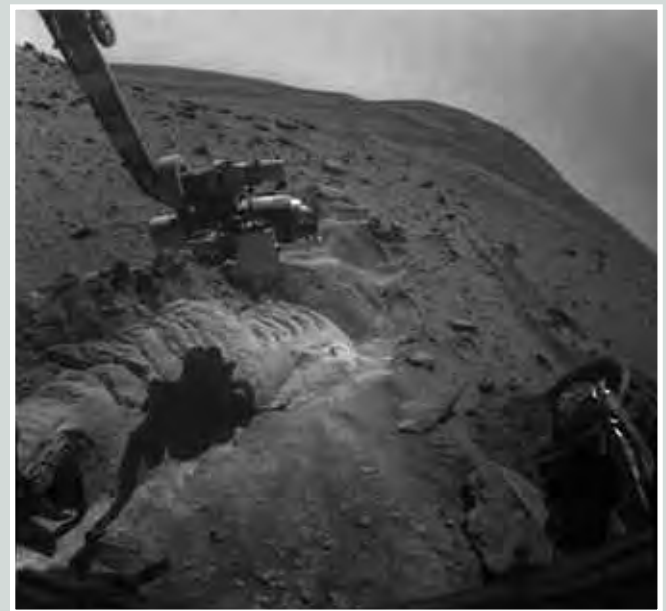
In these Hazcam views after sol 2,154 (January 24, 2010), Spirit sat immobile while NASA announced that the rover was now a stationary lander. In the front view (top), the right-front wheel has remained more or less stationary, acting as a pivot, while the left-front wheel has churned soil as the rover moved. In the rear view (bottom), the two wheels are visible again, though still partially buried.
