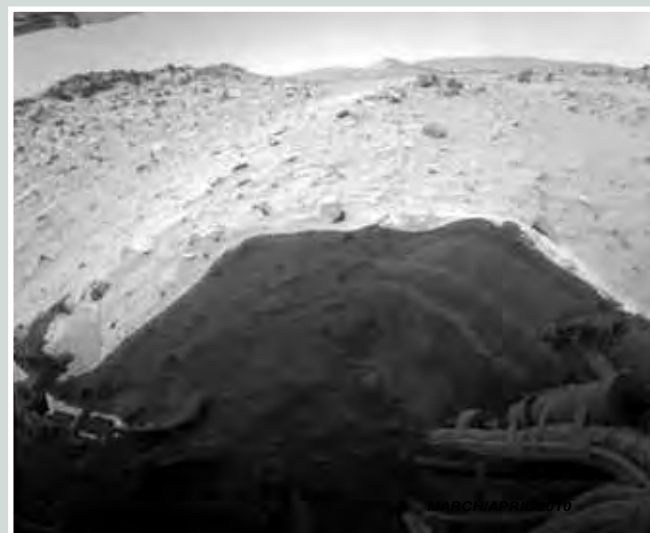
In the front view (top), the immobile right-front wheel sits on the surface while the left-front wheel is nearly totally buried in a large pile of churned-up soil. In the rear view, the rover's two rear wheels should be visible, but both are buried to the rims in Martian soil.
