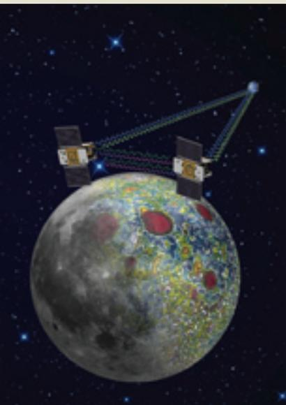
**ABOVE** *GRAIL*'s twin spacecraft used a precision flying technique to map the Moon's gravity field. The probes, launched in September 2011, studied the internal structure and composition of the Moon until December 2012, when mission controllers deliberately crashed them into the lunar north pole.
