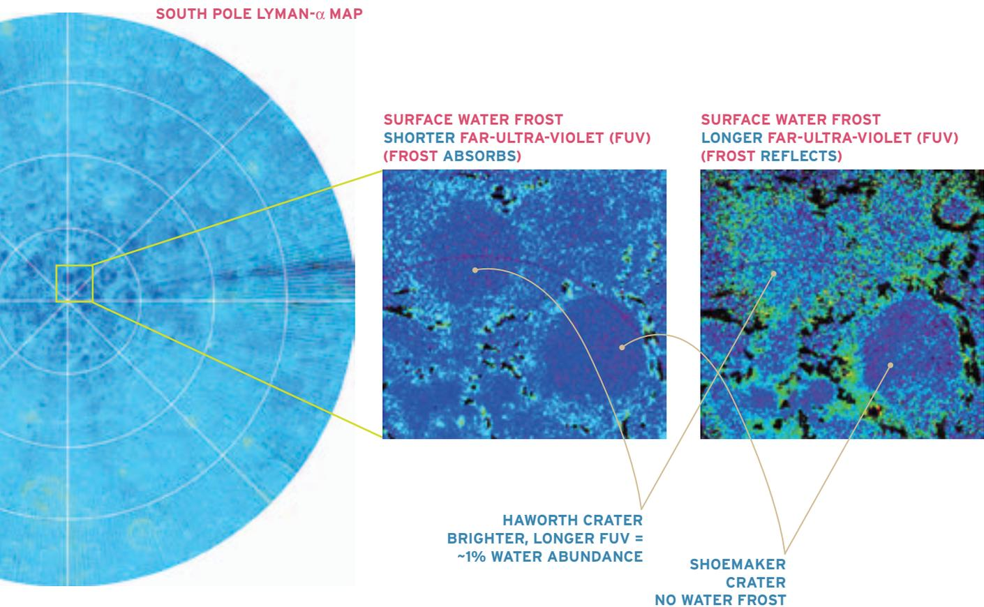
**ABOVE** The Lyman Alpha Mapping Project (LAMP) instrument on Lunar Reconnaissance Orbiter (LRO) has found further evidence of water at the Moon's poles. LAMP has taken measurements inside the permanently shadowed regions there—areas dark enough to hide water and cold enough to keep it stable. The texture of the surface in the PSRs is not well understood, and it adds a layer of complexity to interpretation of the LAMP data gathered there.
