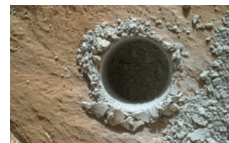
ABOVE The Buckskin drill site on Mars. X-ray diffraction analysis of the Buckskin sample inside the rover's Chemistry and Mineralogy (CheMin) instrument revealed the presence of a silica-containing mineral named tridymite. This is the first detection of tridymite on Mars.
