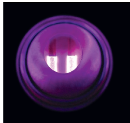
RIGHT Plasma used to generate tholin from a mixture of nitrogen and methane gases.
