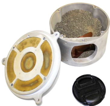
ABOVE PlanetVac Xodiac sampling container following a successful sampling during a Xodiac rocket flight. More than 300 grams (10.5 ounces) of Mars simulant that was collected can be seen in the container. Lens cap for scale.
