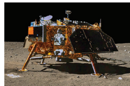
ABOVE This photo of the Chang'e-3 lander was taken by the Yutu rover before the rover's premature failure. The lander is still operating an ultraviolet telescope on the lunar surface more than four years later. Chang'e-4 is nearly the same design, with different science instruments.
