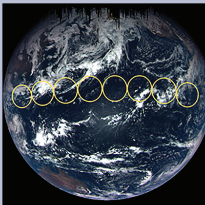
LEFT The OTES instrument gathered its spectral data at nearly the same time that MapCam took this photo. The yellow circles, each 800 kilometers (500 miles) in diameter, show the approximate locations and sizes of the spots on Earth scanned by OTES to produce these curves.
