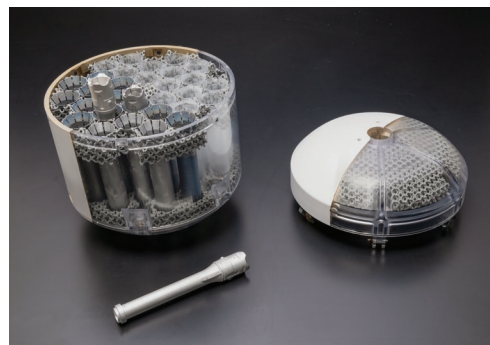
LEFT This image shows a prototype container that could carry Perseverance's sample tubes from Mars back to Earth. Once launched into Mars orbit, the container would be picked up by an orbiting satellite, carried back to Earth, and sent hurtling through Earth's atmosphere to the ground for retrieval.
