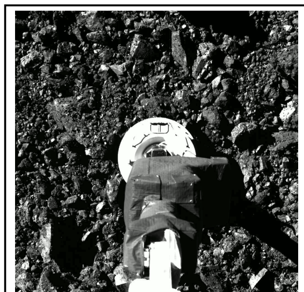
OSIRIS-REx Touch-And-Go (TAG) sample collection event on October 20, 2020 the moment the spacecraft touched down on asteroid Bennu's surface. The sampling event brought the spacecraft all the way down to sample site Nightingale, and the team on Earth received confirmation of successful touchdown at 6:08 pm EDT. Credit: NASA/Goddard/University of Arizona.
