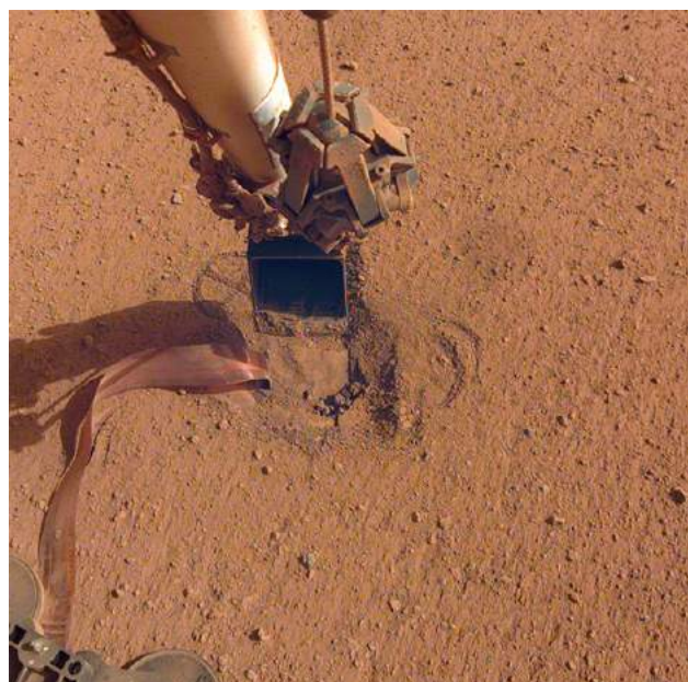
NASA's InSight lander retracted its robotic arm on October 3, 2020, revealing the spot where the self-digging "mole" is attempting to burrow into the planet's surface. It is currently below the surface several centimeters and not visible in this image. Attached to the mole is the copper-colored ribbon, which is laden with temperature sensors designed to measure the heat flow within Mars.
