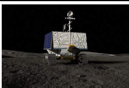
The Volatiles Investigating Polar Exploration Rover (VIPER), shown above, is being sent to the Moon's south pole to sample water ice in the region where the first woman and next man will land under the Artemis Program. Instruments on VIPER are being created by Honeybee Robotics who received their first SBIR award in 2007 and has now graduated from the program.
