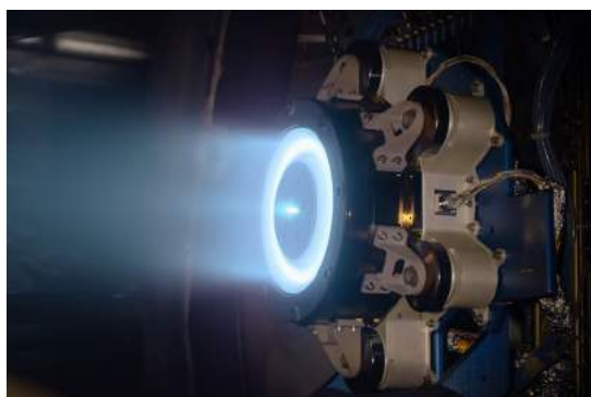
The Electric Propulsion thruster is shown here in testing. The project will be qualifying a 30-50 kilowatt (kW)-class solar electric propulsion system that will be demonstrated on the Lunar Gateway Power and Propulsion Element.
