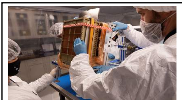
The Near Earth Asteroid (NEA) Scout is the first CubeSat delivered and ready for integration into SLS for the Artemis I mission.
