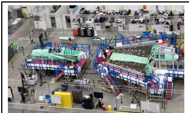
This picture shows the wing and cockpit sections of NASA's X-59 QueSST vehicle coming together at Lockheed Martin's factory in Palmdale, California.
